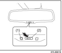
You can adjust the auto dimming rearview mirror by hand so you can see to the rear of your vehicle in the mirror. This rearview mirror has a function of automatically reducing glare from the lights of vehicles behind you. The function works when the ignition mode has been changed to "ON" by pressing the engine switch.
